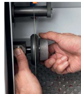
Quick-release nut for T205/T215 Tool-less cut-off wheel change Ref. 51725
