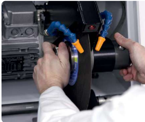
Spindle lock for wheel change with optional quick-clamping nut
