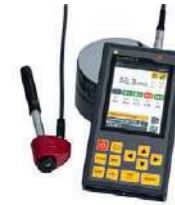
HLD Rebound hardness tester with external probe
