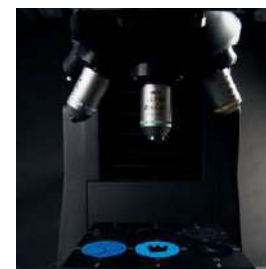
Motorized turret Up to 7 positions, including the touch sensor
