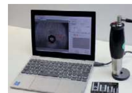
Brinell camera with software for automatic indenter reading and hardness data extraction
