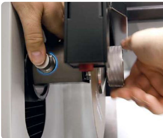
Spindle lock for wheel change with quick-release nut
