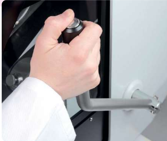
Electromagnetic locking of the cutting arm
