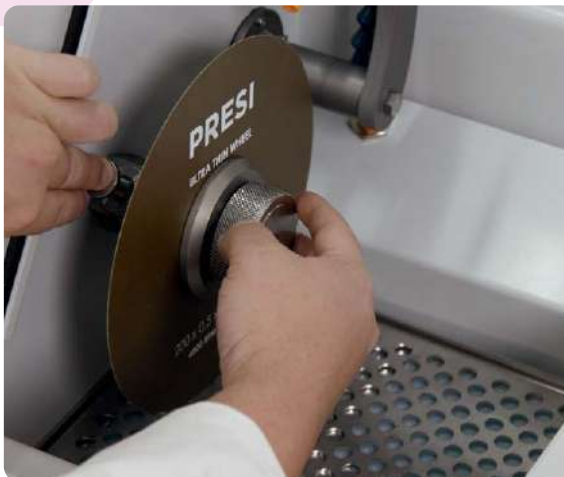
Spindle lock for wheel change with quick-clamping nut option
