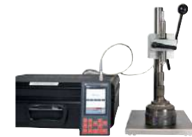
UCI hardness tester mounted on a measuring frame
