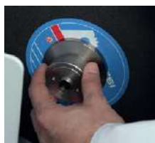
Quick-release nut for Tool-less cut-off wheel change Ref. 51272
