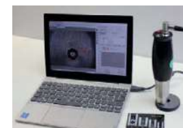
Brinell camera with software for automatic indent reading and hardness data extraction
