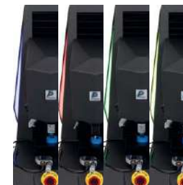
Color code in accordance with the machine status
