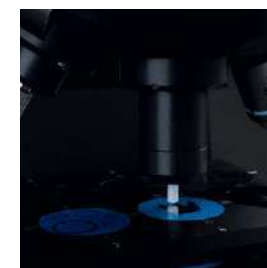
Teflon touch sensor Detects the part without leaving marks and ensures optimal operator safety
