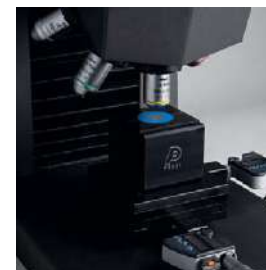
Single sample holder For sample leveling
